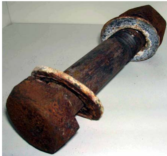
Figure 18: LE spe (Bare + Turn-of-Nut + 120 cycles)
