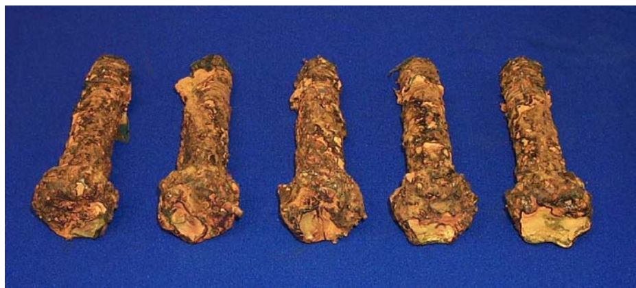
Figure 14: SL std (MG + 5000 hrs per ASTM B117)
