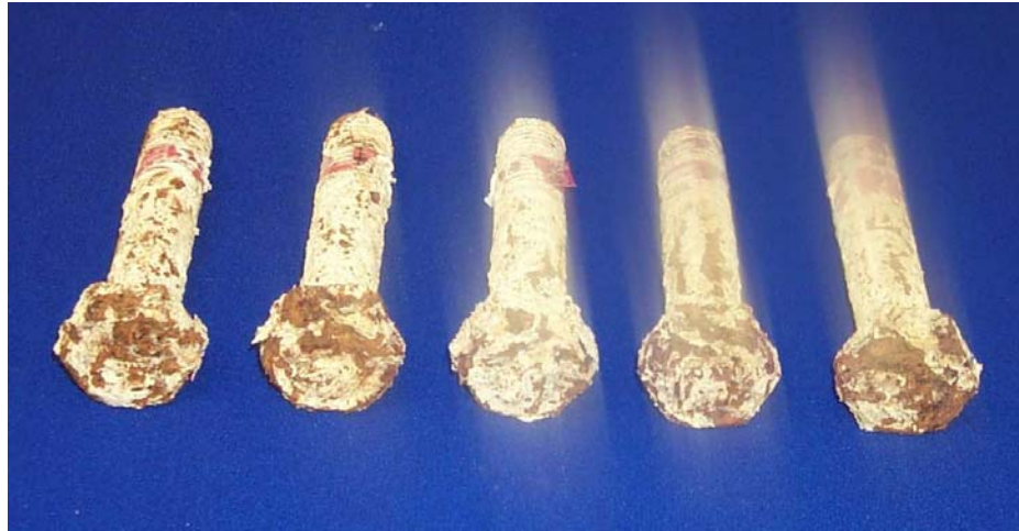
Figure 13: SL std (HDG + 5000 hrs per ASTM B117)
