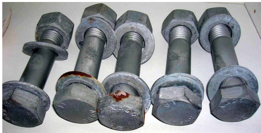
Figure 19: LE spe (DACROMET® + 120 cycles)
