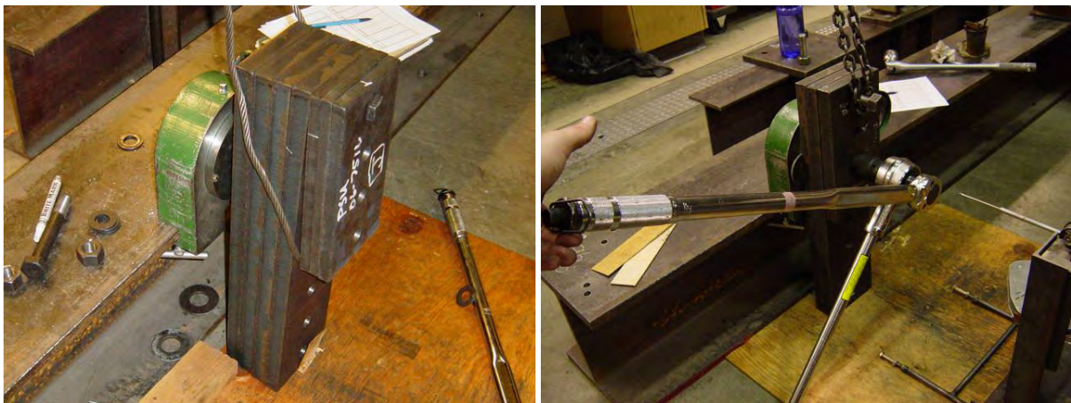
(a) Multi-plate Built-up for Required Thickness (b) Torque Wrench and Torque-multiplier
