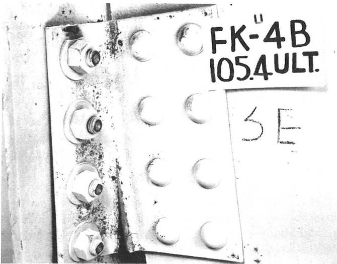
Fig. 18.5. Angle failure in standard beam connection described in Fig. 18.4. (Courtesy of University of Illinois.)
