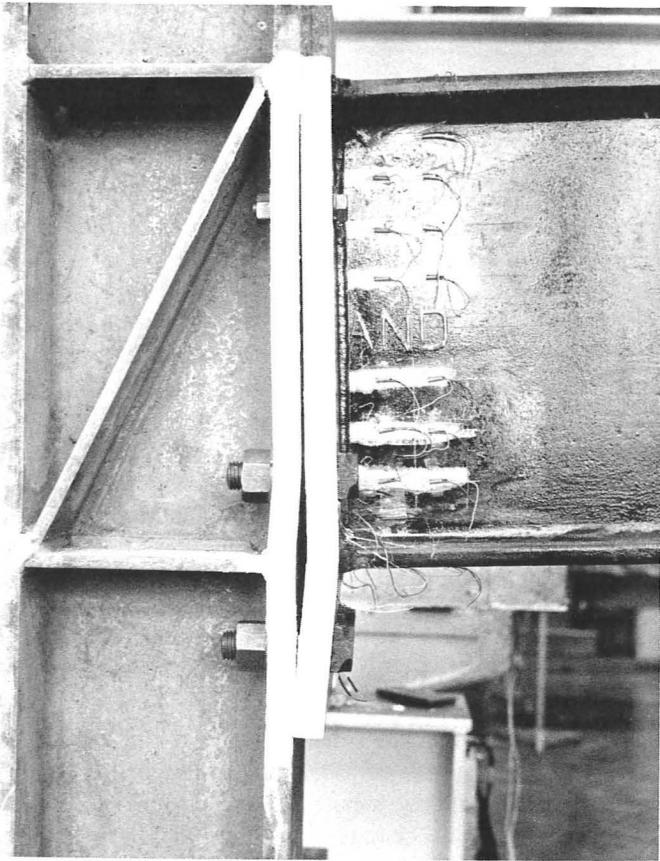
Fig. 18.11. End plate connection after failure. (Courtesy of University of Sheffield).
