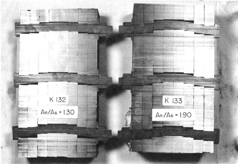
Fig. 5.31. Sawed sections of joints showing bolt bending.
