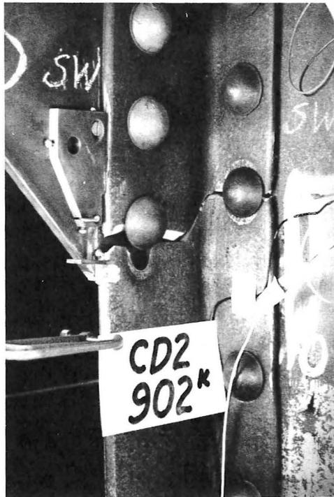
Fig. 6.3. Angle failure in built-up section. (Courtesy of University of Illinois.)
