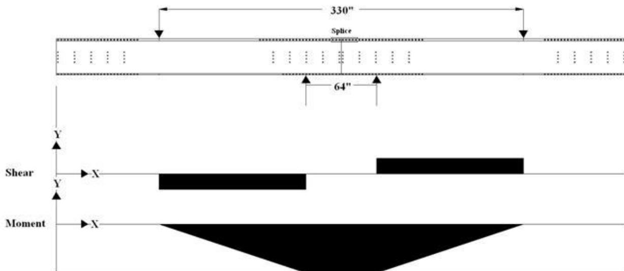
**Figure 19:** Analytical model for girder splice connection.
