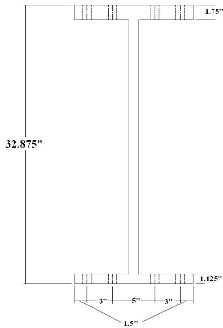
**Figure 16:** Front view of plate girder
