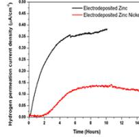
Permeation transients of Zn and Zn-Ni coatings on low carbon steel shim
