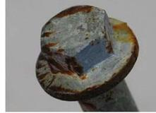
Stress corrosion cracking
