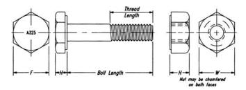
Figure C-2.2. Heavy-hex structural bolt and heavy-hex nut.
