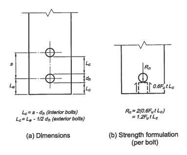
*Figure. C-5.1. Bearing strength formulation.*
