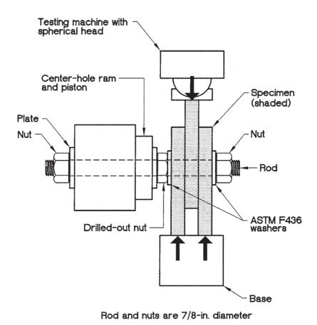
Figure A-3. Compression slip test setup.
