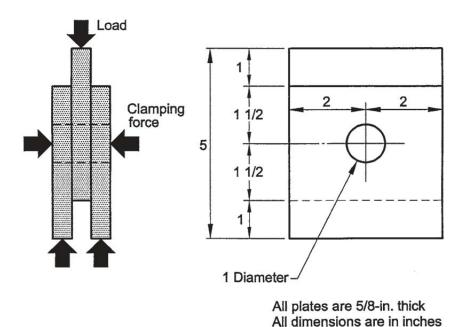
Figure A-1. Compression slip test specimen.
