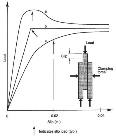
Figure A-4. Definition of slip load.
