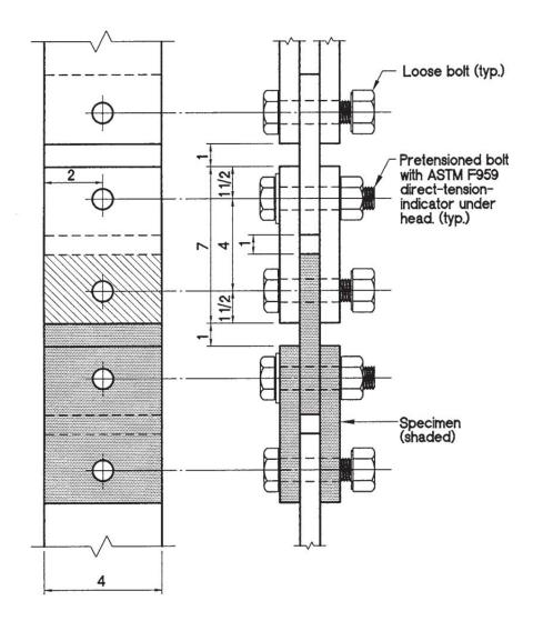
All dimensions are typical All plates are 5/8-in. thick All dimensions are in inches
