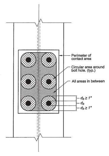
Figure C-3.1. Faying surfaces of slip-critical connections painted with unqualified paints.
