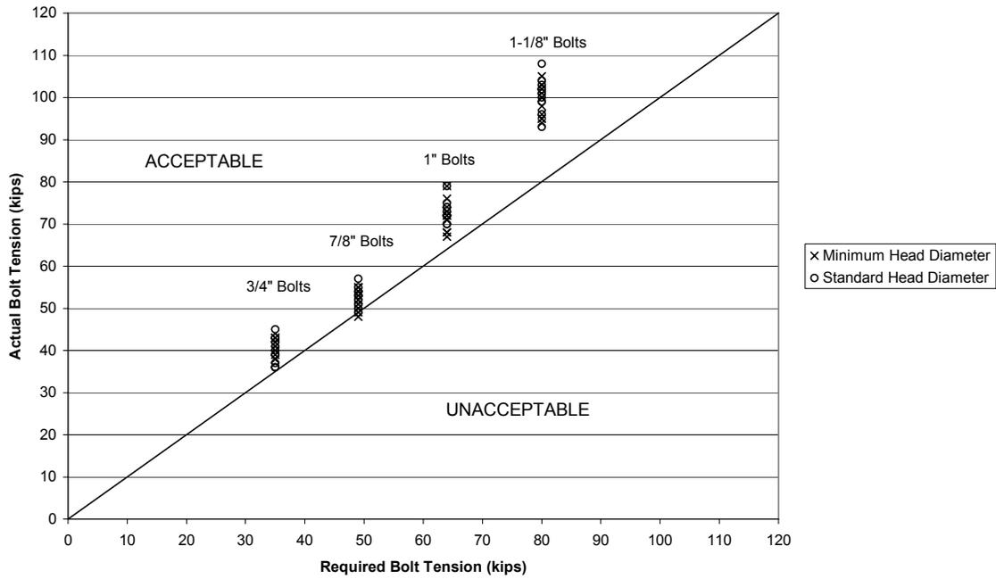
**Figure 5.5: A490 Strength, Centered Bolts, Oversized Holes**
