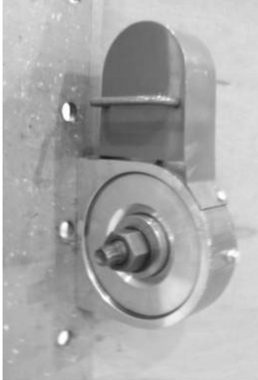
**Figure E.1: Rear View of Typical Skidmore Setup**
