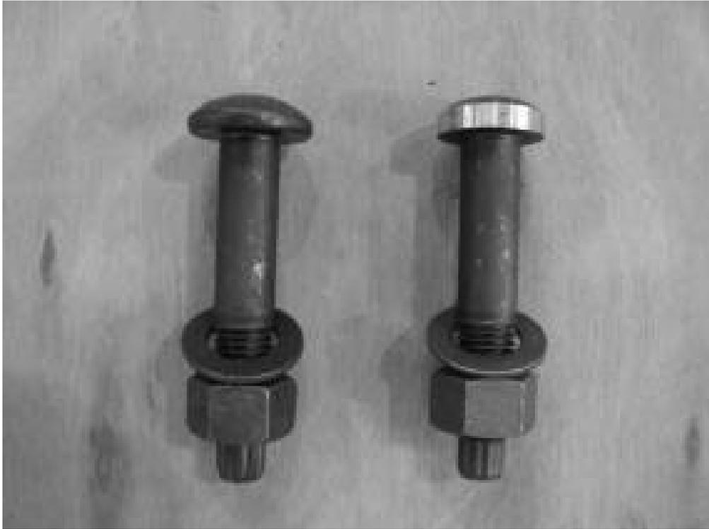
**Figure 3.1: Photo of Manufacturer's Standard and F1852 Minimum Diameter 1-1/8" Bolts**
