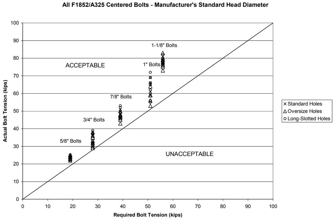
**Figure C.2: All F1852/A325 Strength, Centered Bolts, Standard Head**
