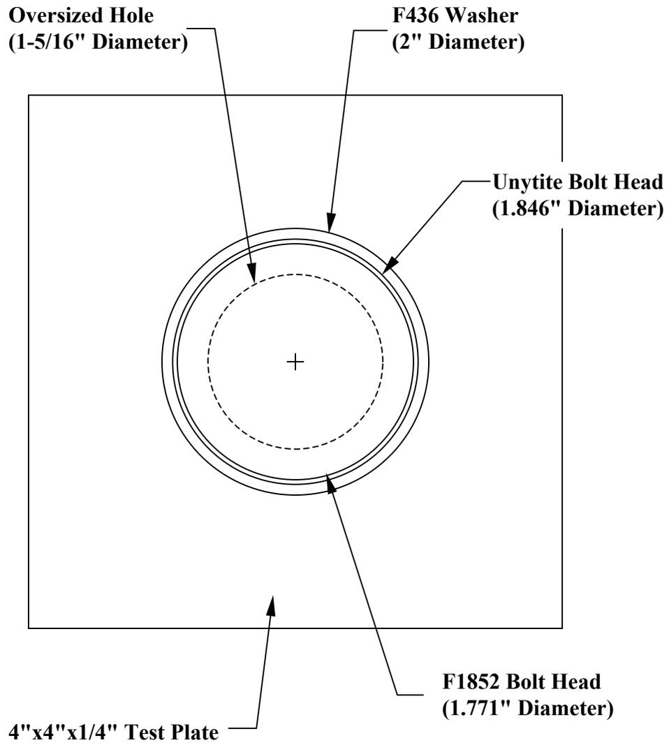
**Figure B.2: Bolt and Plate Layout for 1" Bolt in Oversized Hole**
