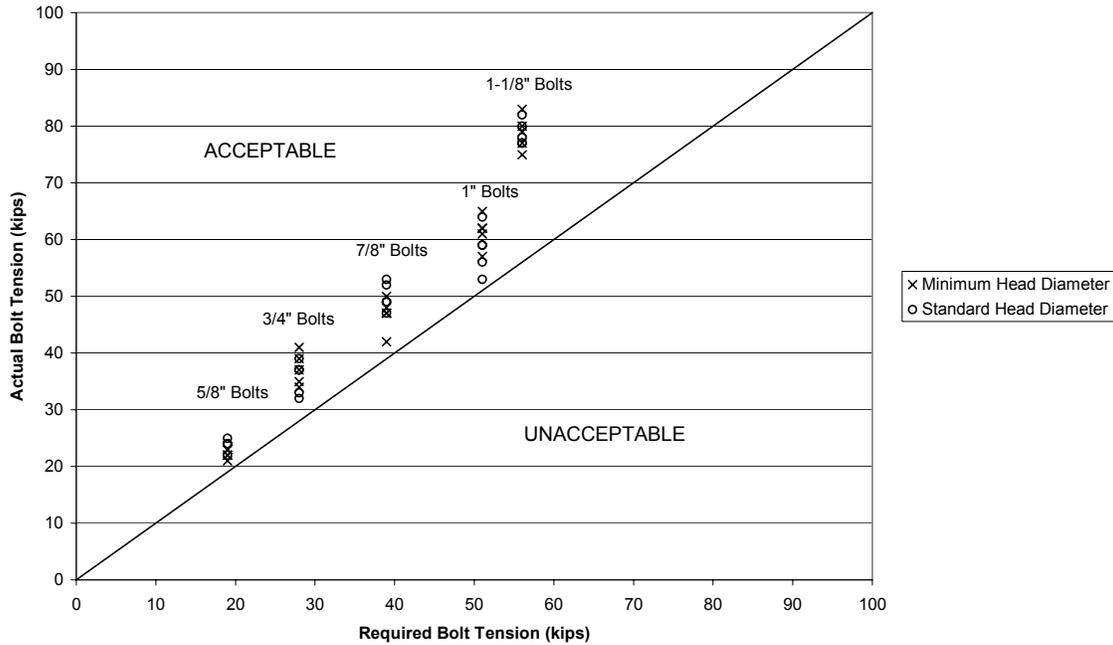
**Figure 5.3: F1852/A325 Strength, Centered Bolts, Long-Slotted Holes**
