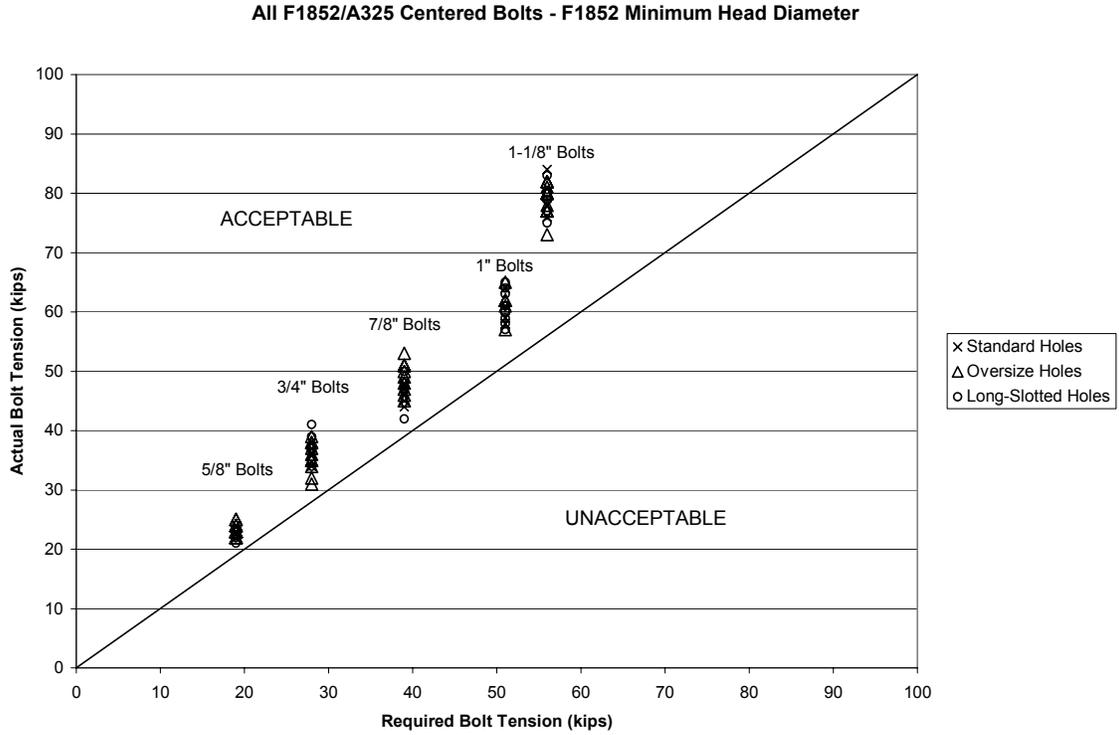
**Figure C.1: All F1852/A325 Strength, Centered Bolts, Minimum Head**
