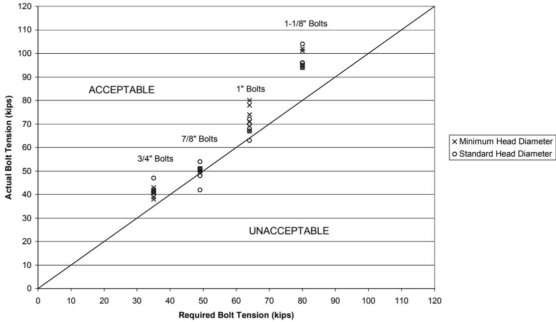
**Figure 5.4: A490 Strength, Centered Bolts, Standard Holes**
