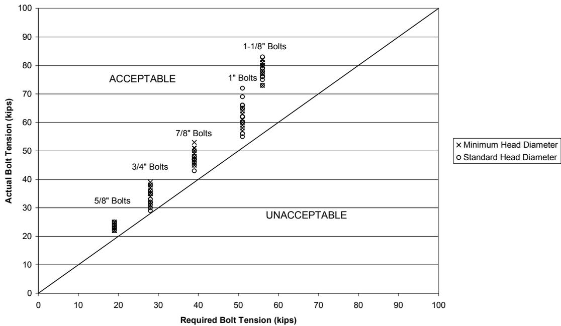
Figure 5.2: F1852/A325 Strength, Centered Bolts, Oversized Holes
