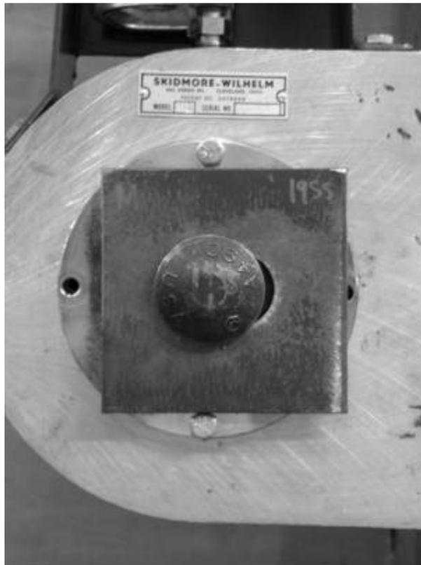
**Figure E.4: Setup for 1" Bolt, A490 Strength, Off-Centered Test**
