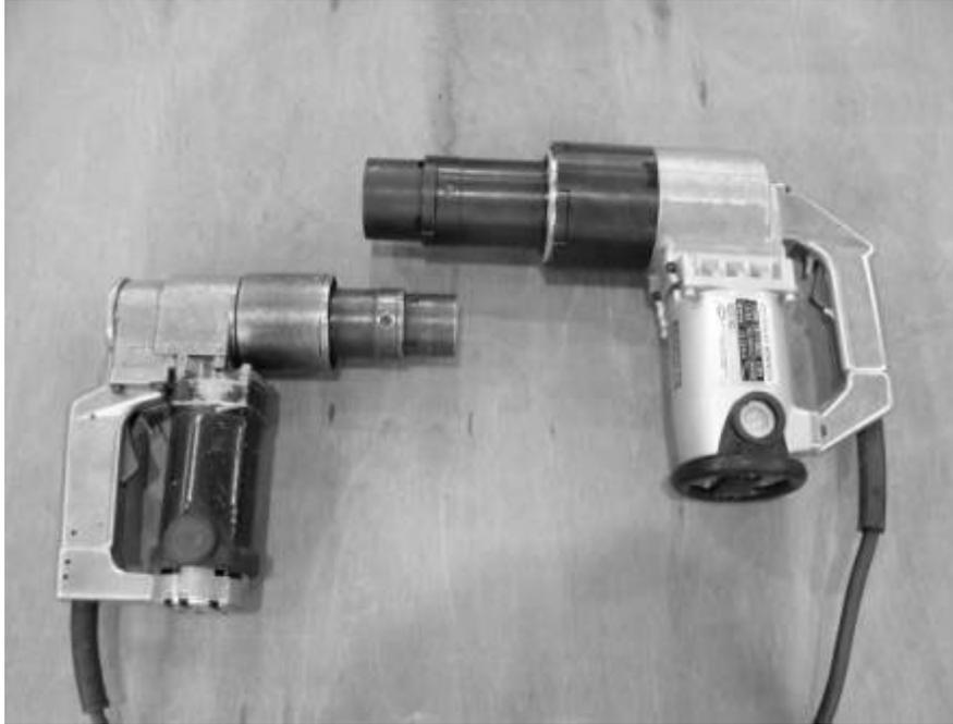
**Figure E.3: Torque Wrenches Used for Tightening**
