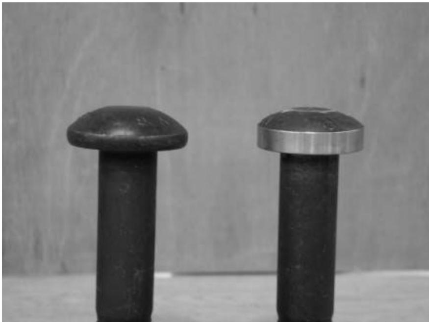
**Figure E.2: Manufacturer's Standard and F1852 Minimum Bolt Heads**
