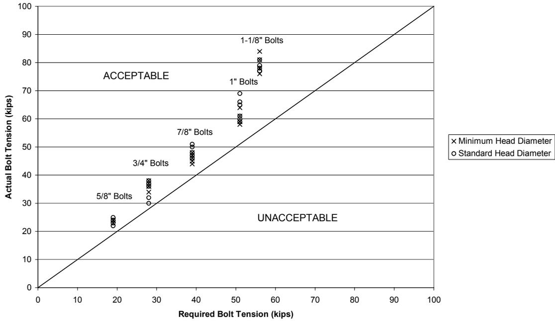
Figure 5.1: F1852/A325 Strength, Centered Bolts, Standard Holes
