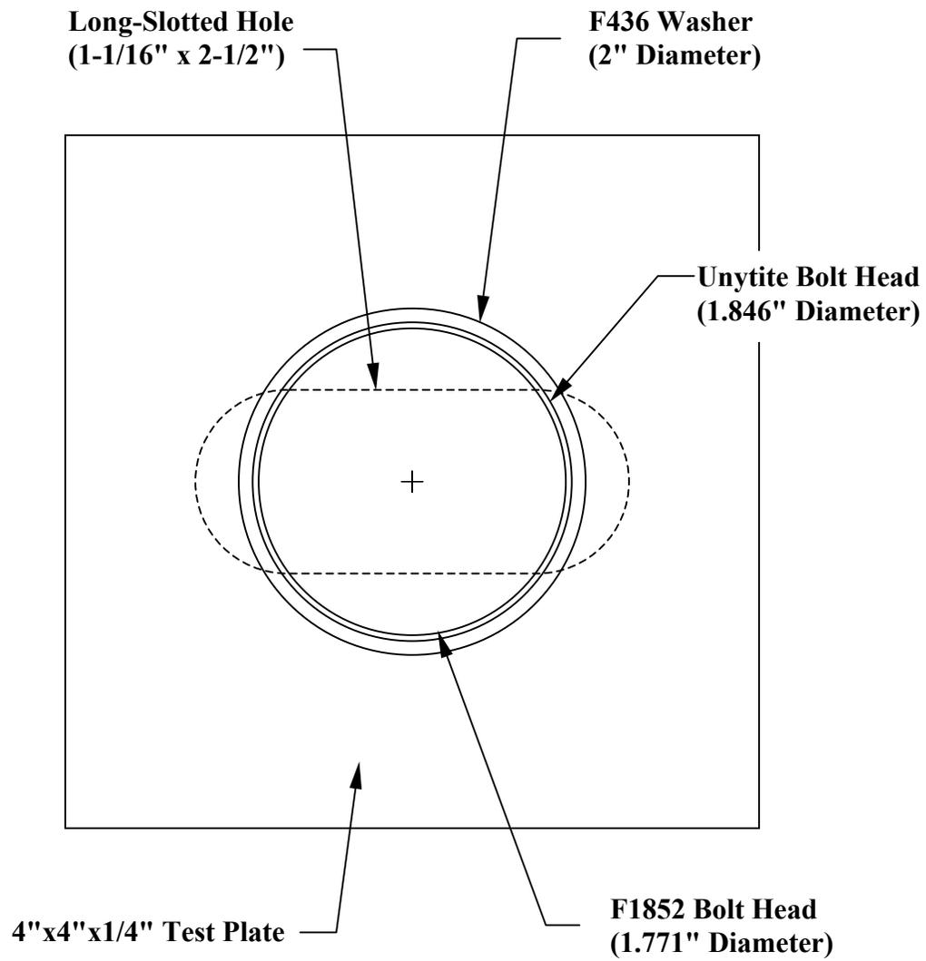
**Figure B.3: Bolt and Plate Layout for 1" Bolt in Long-Slotted Hole**
