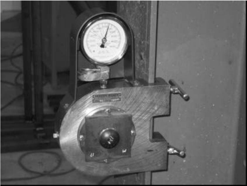
**Figure 4.1: Typical Skidmore Setup with Test Sample**
