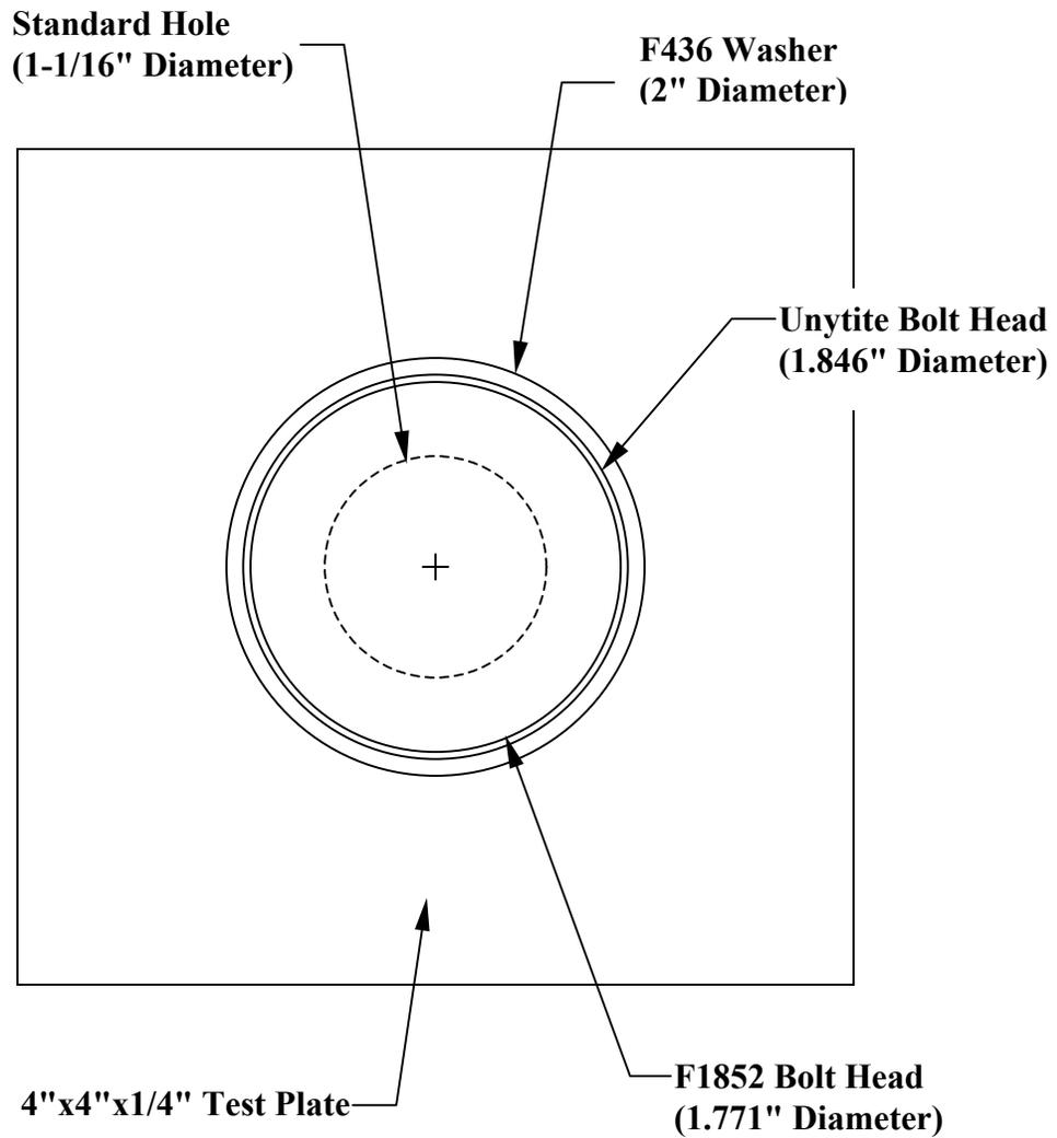
**Figure B.1: Bolt and Plate Layout for 1" Bolt in Standard Hole**
