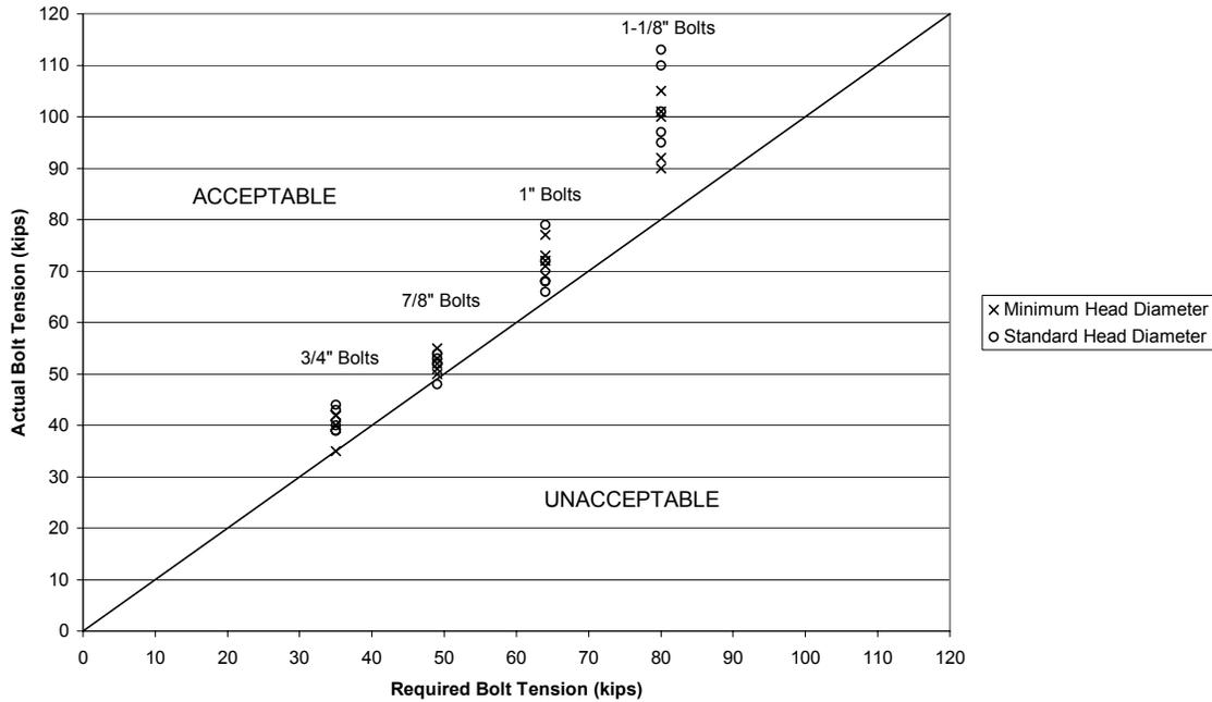
**Figure 5.6: A490 Strength, Centered Bolts, Long-Slotted Holes**
